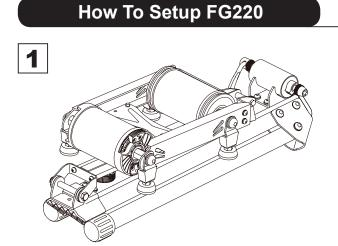
FG220 is folded into three in the package. Set in this style when stored.
