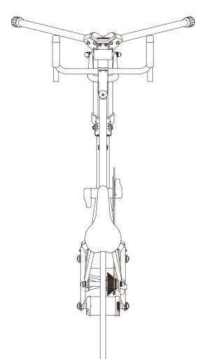
It's normal for the rear tire to sway or move back and forth slightly when in use. As long as the tire doesn't touch the sides of the rollers this is ok.
