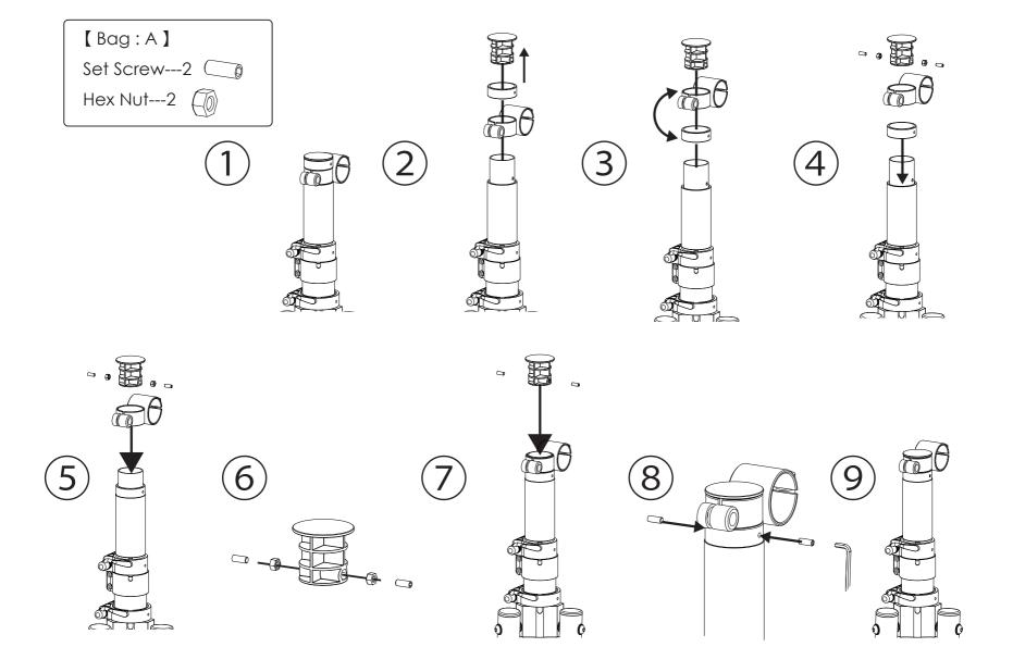
**4.** Before inserting the Right Arm Clamp int o its Receptacle, apply the provided, packaged (white) Grease to the inside of the Clamp Receptacle, and on the outside of the Clamp's rotating surface.
