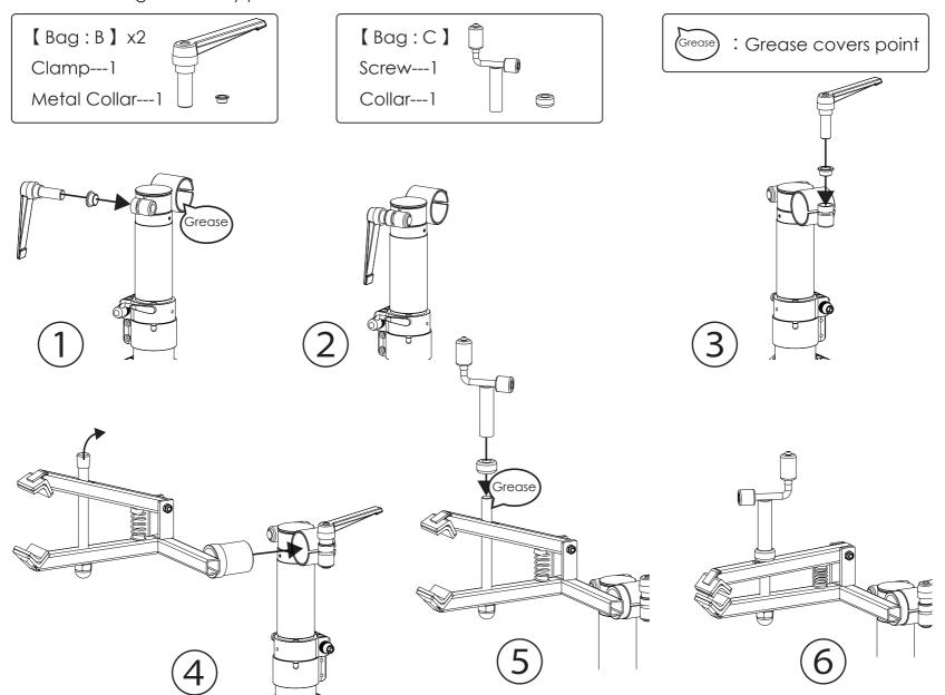
**5.** Adjust the Right Arm Clamp's rotation by loosening the Indexable Locking Lever. Move to the desired position, then tighten the Locking lever firmly! We recommend this step only be done without a bicycle in the stand.
