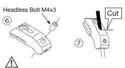
Simply cutting the Stay can still be dangerous because the cut surface is very sharp. Grind it for your safety.
