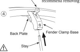
Set the positions of the fender and Clamp Base properly so they do not interfere with the spinning wheel or tire. If the fender gets caught in the wheel while riding, it may cause a sudden stop and could result in an injury.
