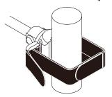
Place the pad on the frame, then wrap the tape around the tube.
