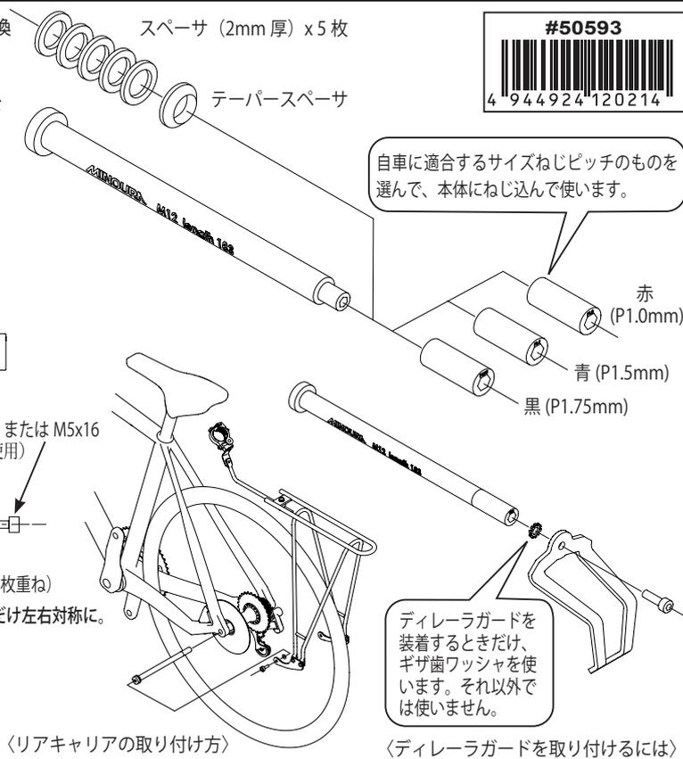
The perfect set of 12mm thru axle for installing front racks. With so many thru axle specs on the market this set fixes the issues of fit by including three different thread pitch sizes in in one set.
